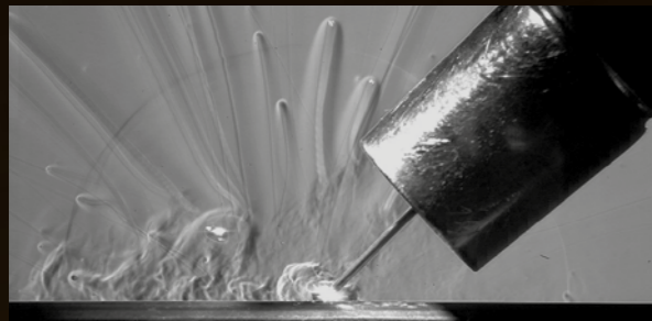
Schlieren imaging of arc welding – With front-illumination
